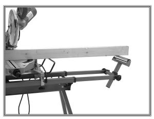
Figure 6. Adjusting the support rollers.
